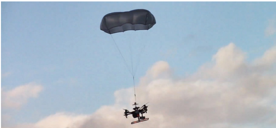
Figure 2. NUAIR parachute system
